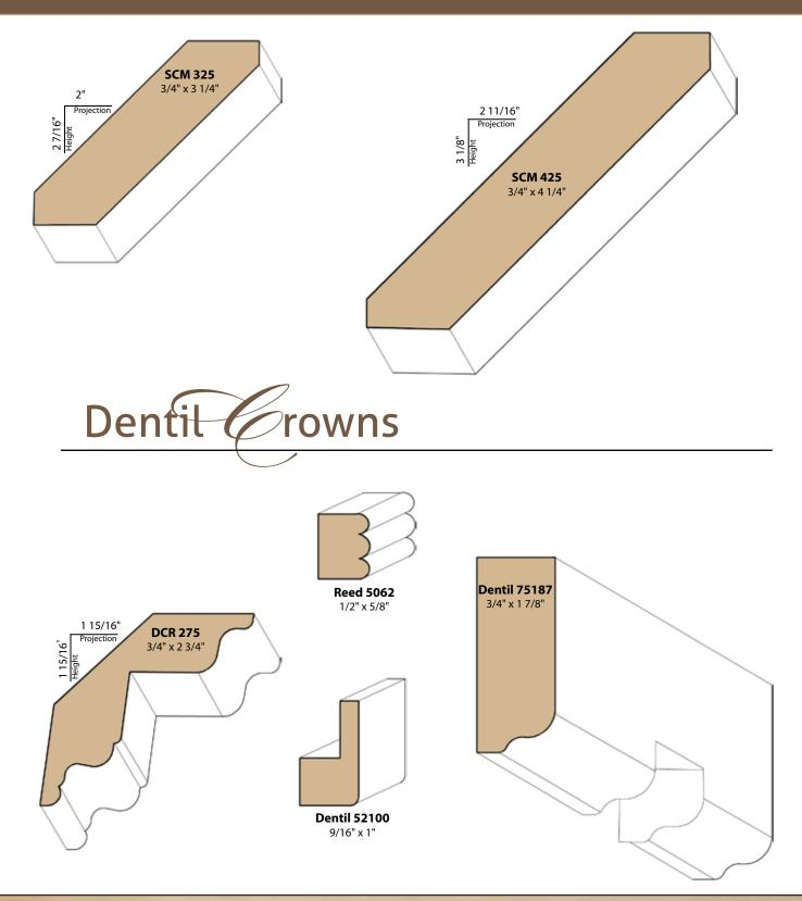
Series of small square blocks evenly spaced and projecting like teeth as used in cornice, front entrances, crossheads and mantels.
